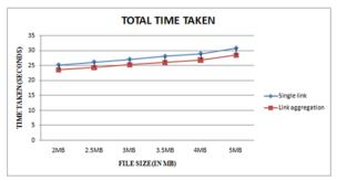
Figure 6: Total time taken for both link aggregation and single link using UDP.
