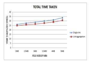
Figure 8: Total time taken for both link aggregation and single link using SCTP.
