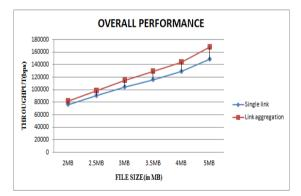
Figure 9: Overall performance of link aggregation and single link using SCTP.
