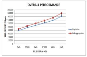
Figure 7: Overall performance of link aggregation and single link using UDP.
